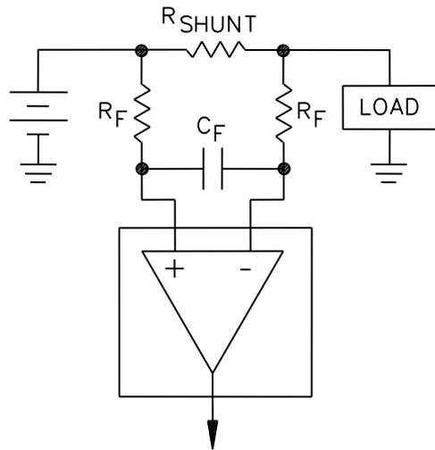
FIGURE 5. Input filter circuit.
