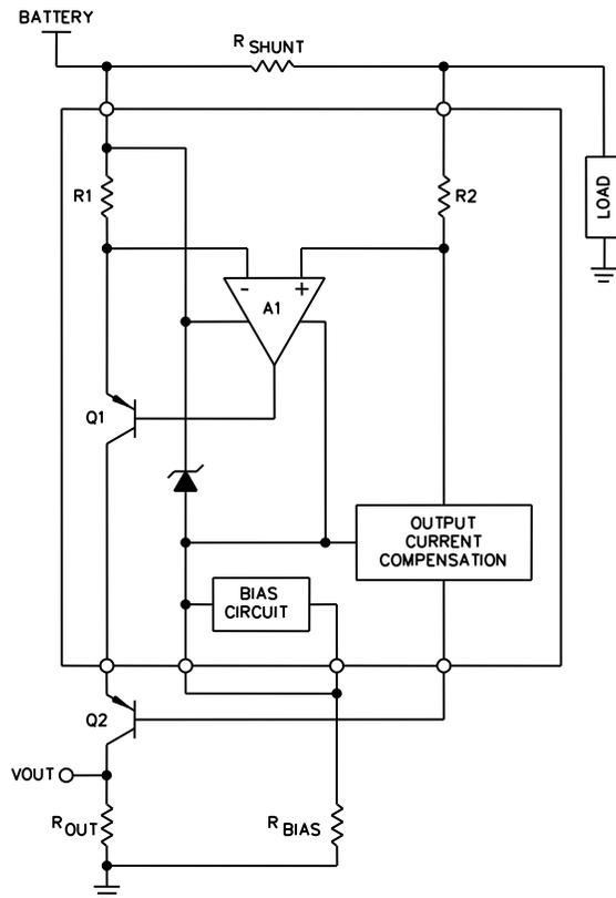
FIGURE 4. High voltage external PNP configuration circuit.
