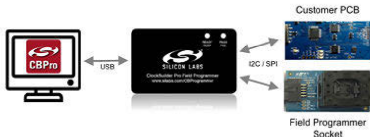
Figure 4.1. PC to CBPROG-DONGLE Connection
