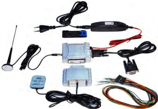
The image shows the components of the HB20 bundle: the HB10 bundle components plus a small blue GPS add-on board, a GPS antenna on a cable, and a multi-colored I/O extension cable.
