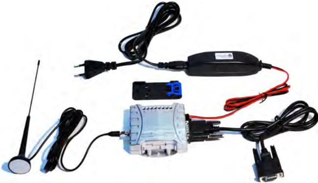
The image shows the components of the HB10 bundle: a central white industrial unit, a black magnetic antenna on a cable, a black power supply unit with a power cord, a blue serial cable, a black Din clip, and a black softtool.
