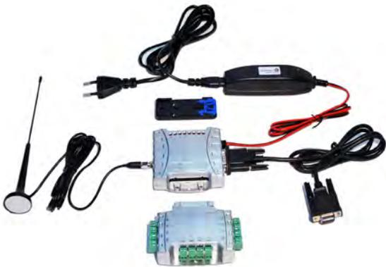
The image shows the components of the HB30 bundle: the HB10 bundle components plus a green I/O add-on board.
