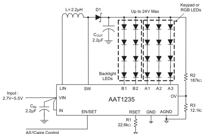
**High Efficiency White LED Drivers for Backlight and Keypad**
