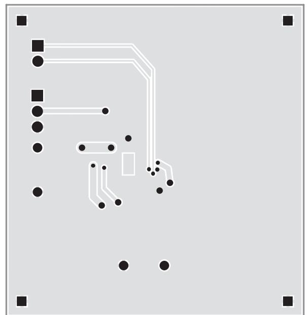
**Figure 5: AAT1235 Evaluation Board Bottom Side Layout.**
