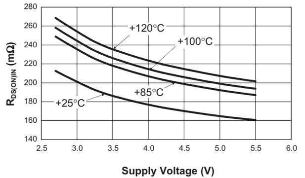
**Low Side Switch On Resistance vs. Supply Voltage and Temperature**
