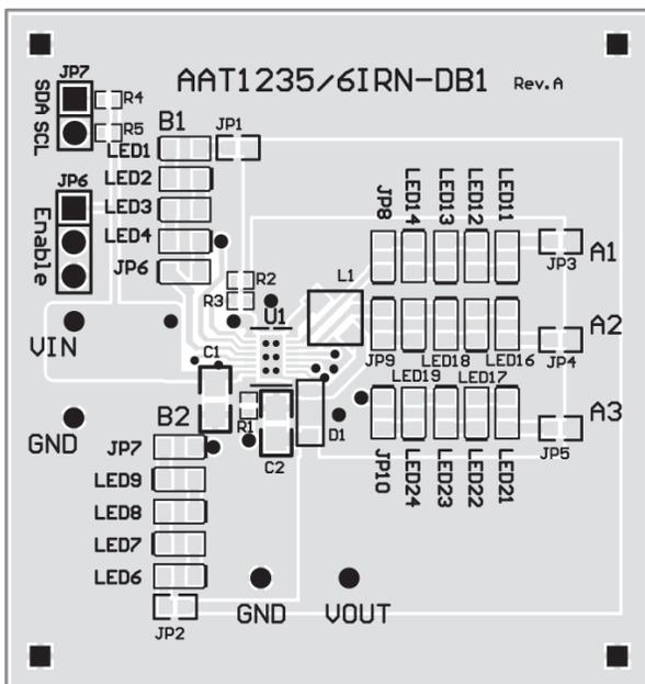
**Figure 4: AAT1235 Evaluation Board Top Side Layout.**
