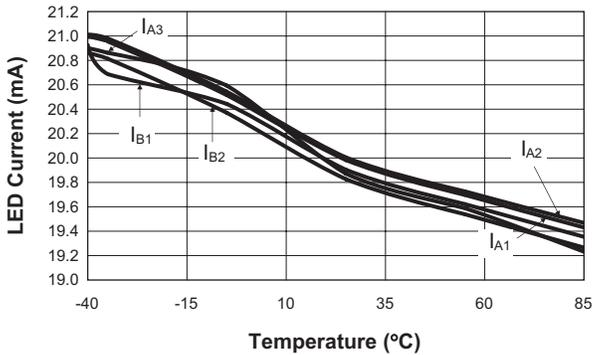
**LED Current Accuracy vs. Temperature**
