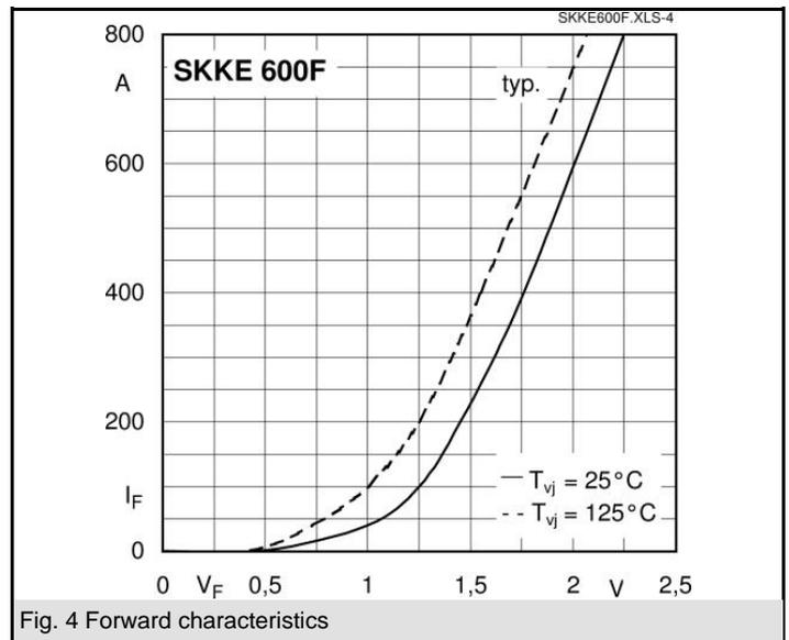
Fig. 4 Forward characteristics
