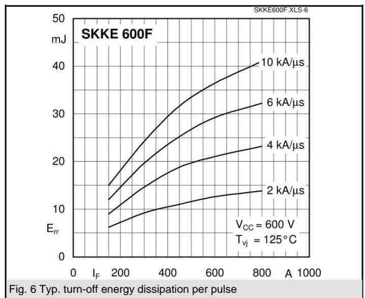
Fig. 6 Typ. turn-off energy dissipation per pulse
