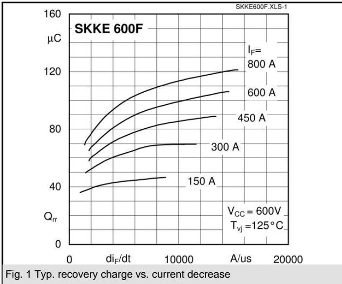
Fig. 1 Typ. recovery charge vs. current decrease
