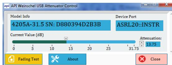
API Weinschel's LabView based USB Control Center Software (AUCS) can also be used in the operation of this series of digital attenuators. The AUCS will allow the user to setup, control, and perform test and measurements over a standard USB 2.0 communication interface. Additional information is available in the Operating & Installation Manual, IM-611.
