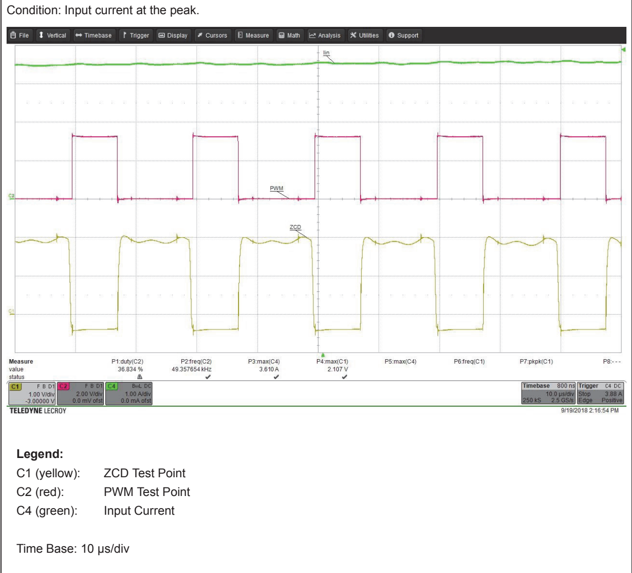
FIGURE 1-10: ZERO-CROSS DETECTION (ZCD), PWM TEST POINTS
