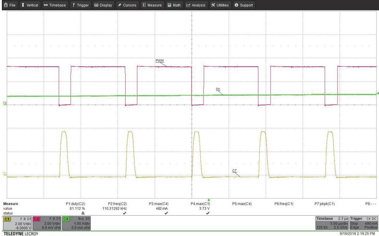
FIGURE 1-9: ZERO-CROSS DETECTION (ZCD), PWM TEST POINTS
