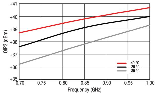
Figure 14. OIP3 vs Frequency Over Temperature
