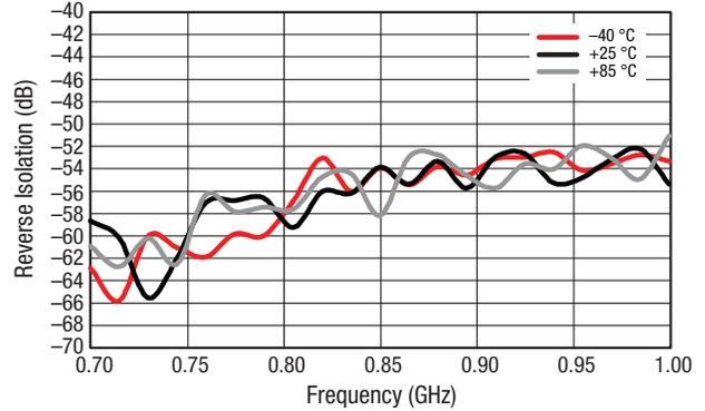
Figure 6. Reverse Isolation vs Frequency Over Temperature, Narrow Band
