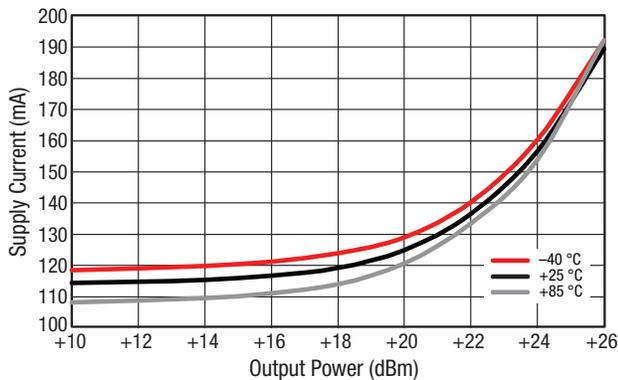
Figure 17. Supply Current vs Output Power Over Temperature
