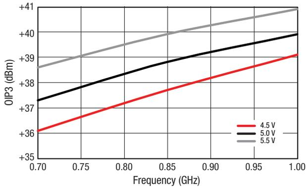
Figure 15. OIP3 vs Frequency Over Voltage
