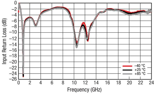
Figure 9. Input Return Loss vs Frequency Over Temperature, Wide Band
