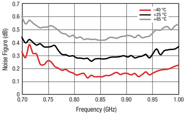
Figure 3. Noise Figure vs Frequency Over Temperature
