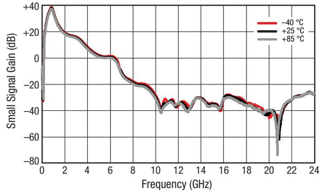
Figure 8. Small Signal Gain vs Frequency Over Temperature, Wide Band
