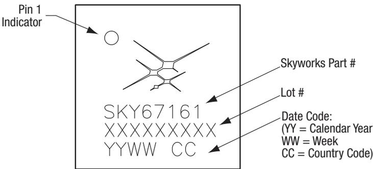
Figure 21. Typical Case Markings (Top View)
