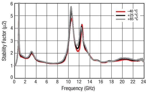
Figure 13. Stability Factor ( $\mu_2$ ) vs Frequency Over Temperature
