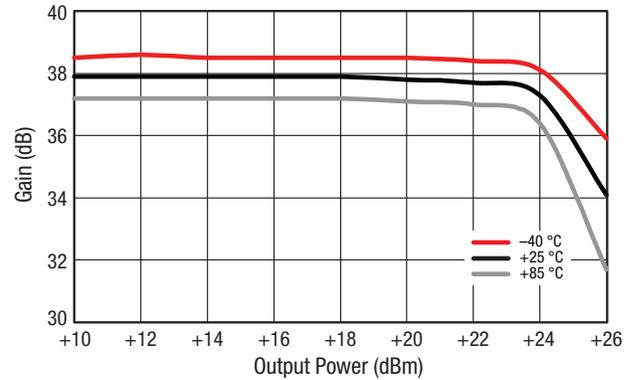
Figure 16. Gain vs Output Power Over Temperature
