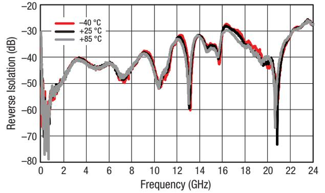
Figure 10. Reverse Isolation vs Frequency Over Temperature, Wide Band
