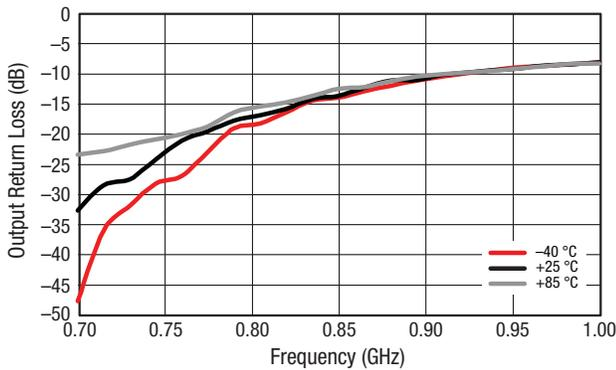
Figure 7. Output Return Loss vs Frequency Over Temperature, Narrow Band
