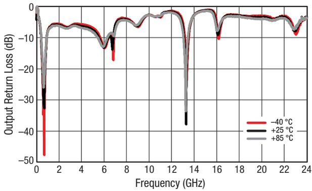
Figure 11. Output Return Loss vs Frequency Over Temperature, Wide Band
