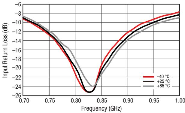
Figure 5. Input Return Loss vs Frequency Over Temperature
