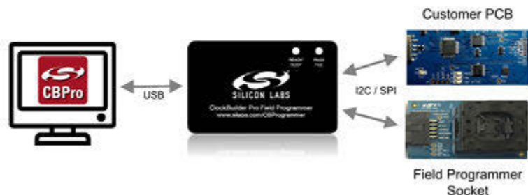
Figure 4.1. PC to CBPROG-DONGLE Connection
