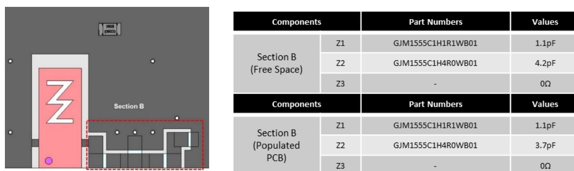
Figure 13 – DUO mXTEND™ (NN03-320) PCB layout for GNSS (left). BoM of DUO mXTEND™ matching network for GNSS (1561 – 1606MHz) in a Free-Space PCB (right top). Adjusted BoM of matching network for GNSS (1561 – 1606MHz) when casings and electronics are present (right bottom).
