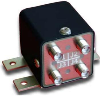
The CS-37 Failsafe Switch is a long-life high performance transfer switch designed for use in 50 Ohms coaxial transmission lines operating over frequencies ranging from DC to 18 GHz. The switch is designed for minimum size compatible with SMA connector spacing.
