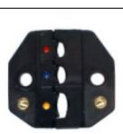
0.5 to 6 sq.mm. AWG 22-18, 16-14, 12-10 For insulated terminals from
