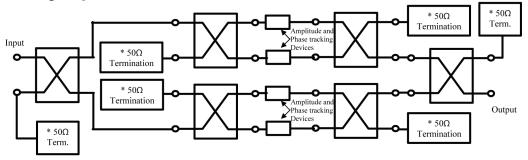
The splitter/combiner networks illustrated above use only 3dB (hybrid) couplers and are limited to binary divisions (2 number of splits, where n is an integer). Splitter/combiner circuits configured this way are known as "corporate" networks. When a non-binary number of divisions is required, a "serial" network must be used. Serial networks can be designed with [3, 4, 5, ....., n] splits, but have a practical limitation of about 8 splits.
