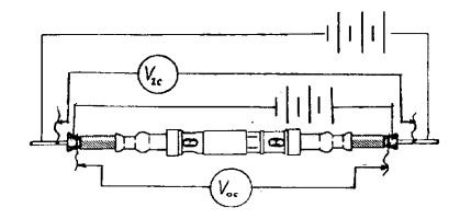
Note: a) Measure voltage drop at specified current and calculate resistance.
