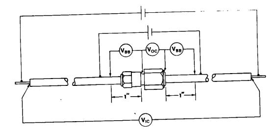
NOTE: (a)  $V_{BB}$  is shield to body measurement.  $V_{OC}$  is outer contact measurement.  $V_{IC}$  is inner contact measurement.
