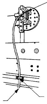
Connector mounted to rotating fixture using normal mounting hardware. (Connector not mated with its counterpart)
