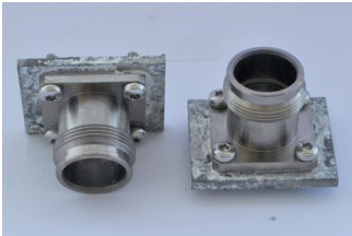
Figure 7 Corrosion of samples after 720 hrs salt mist test on aluminium (without insulation)
