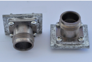
Figure 7 Corrosion of samples after 720 hrs salt mist test on aluminium (without insulation)
