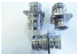
Figure 6 Corrosion of samples after 720 hrs salt mist test.
