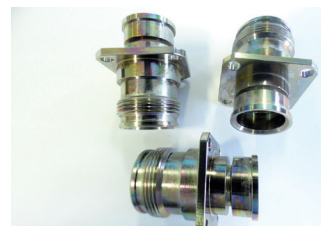
Figure 6 Corrosion of samples after 720 hrs salt mist test.
