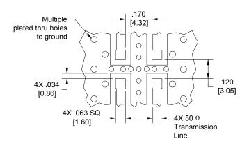
Dimensions are in Inches [Millimeters] JP510 Rev A Mounting Footprint
