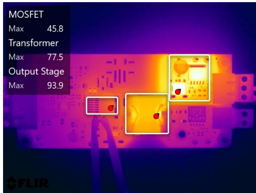
Figure 10: Thermal Image at Steady-Stage V_{in}=60V , I_{out}=1.2A
