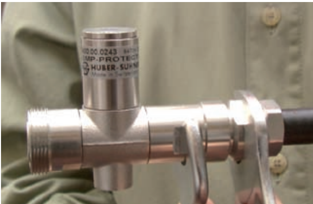
Coupling nut torque forces must not exceed IEC standard or manufacturer detail specifications (IEC: DIN 7/16 - 30 Nm (22.1 ftlb) max. and N - 1.13 Nm (0.8 ftlb) max.).
