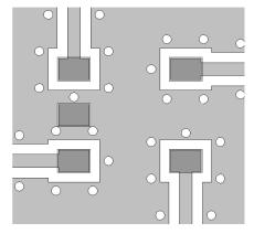
Recommended PCB layout shown above uses 1.6 mm FR4, rounded coplanar wave guide, transmission line width 0.70 mm and gap 0.57 mm.
