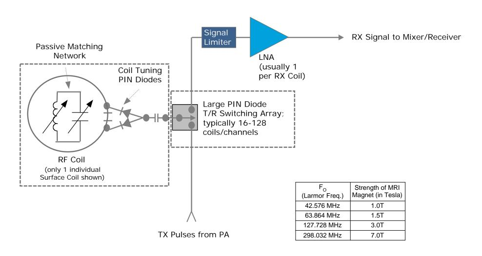
Non-magnetic components are often specified for this section of the overall MRI system.
