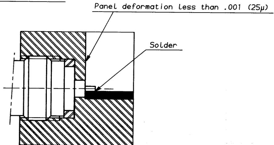
Assemble metal gasket onto connector. Screw both parts into the housing.
