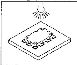
Please follow RADIALL's recommended temperature profile . This profile can be used with Infra - red reflow , Vapor phase soldering and Forced air convection .
