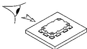
Verify by visual inspection that component is centred on the mounting pads .
