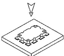
For small, lightweight components such as chip components, a self-alignment effect can be expected if small placement errors exist. However, this effect is not as expected for couplers components and they require precise positioning on their soldering pads; typically ± 0.25 mm.
