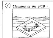
When using a conventional solder cream with high level of residue, please clean the PCB with a substitute product, similar to CFC, that complies to the International Environment Agency rules. It is important to do the cleaning operation step less than fifteen minutes after reflow.
