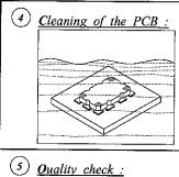
When using a conventional solder cream with high level of residue, please clean the PCB with a substitute product, similar to CFC, that complies to the International Environment Agency rules. It is important to do the cleaning operation step less than fifteen minutes after reflow.
