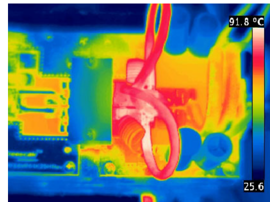
98 MHz, 1100 W CW, 78% Drain Efficiency
