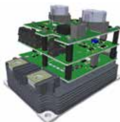
XIFM Intelligent Plug-and-Play 3.3 kV Gate Driver
