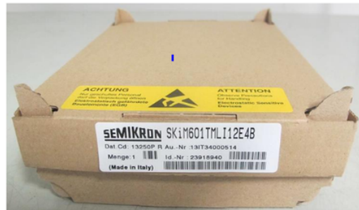
Figure 1 Current carton box packaging and plastic blister for SKiM®4 currently delivered without pre-applied TIM
