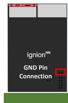
Figure 34 - Connection at 57 mm on the opposite side of the antenna.
