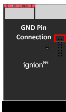
Figure 32 - Connection at 19 mm on the opposite side of the antenna.
