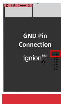
Figure 33 - Connection at 38 mm on the opposite side of the antenna.
