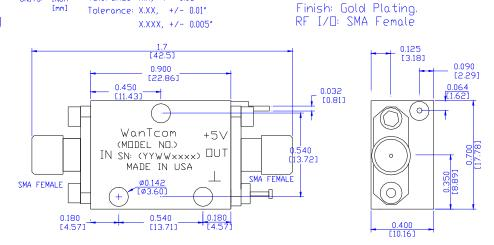
For the pin type input and output application, remove the input and output SMA connectors.
