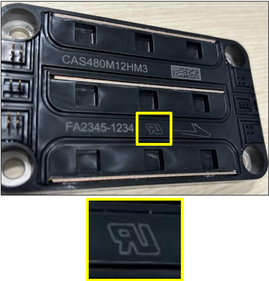
Figure 1. Laser marking on the power modules which shows it is covered under the UL Component Recognition Program.
