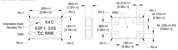
Dimensions are in Inches [Millimeters] X4C50F1-30S Mechanical Outline
