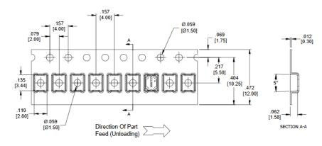
Example of Tape and Reel packaging with the "R" suffix
