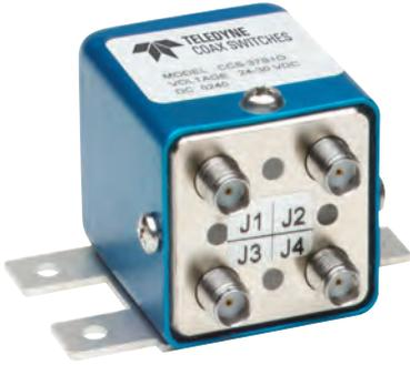
The CCS-37 Failsafe Switch is a long-life high performance transfer switch designed for use in 50 Ohms coaxial transmission lines operating over frequencies ranging from DC to 18 GHz. The switch is designed for minimum size compatible with SMA connector spacing.
