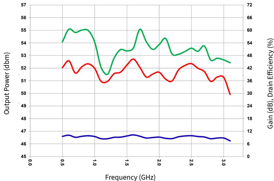
Figure 8. Output Power, Power Gain, and Drain Efficiency vs Frequency of Two CG2H30070F Combined as Measured in the Combined Demonstration Amplifier CG2H30070F-AMP2 with Couplers
