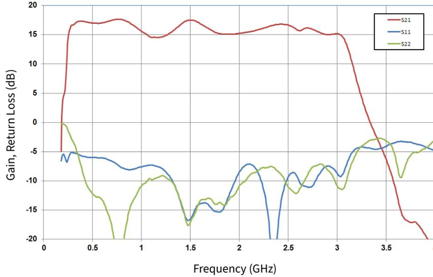
Figure 1. Small Signal Gain and Return Losses of the CG2H30070F vs Frequency as Measured in the Single-ended Demonstration Amplifier CG2H30070F-AMP
