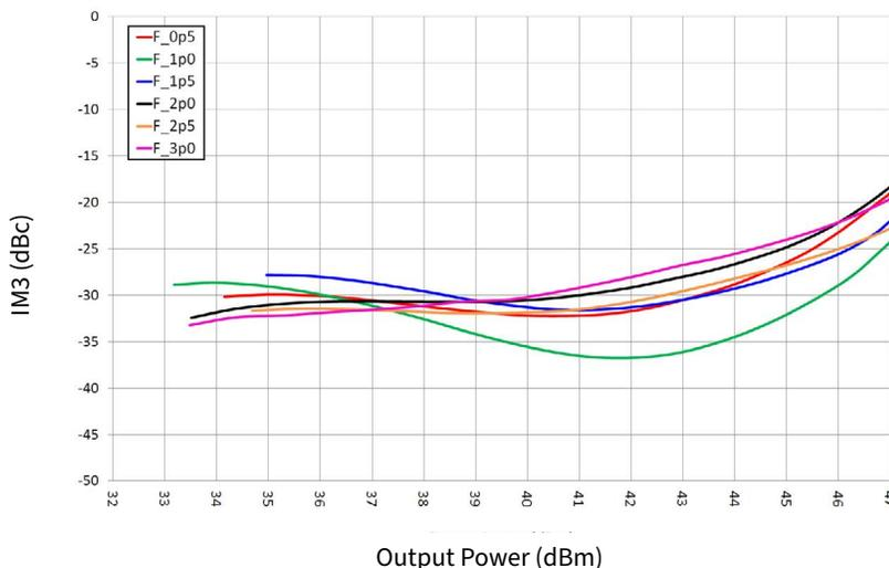
Figure 6. IM3 vs Output Power of the CG2H30070F as Measured in the Single-ended Demonstration Amplifier CG2H30070F-AMP
