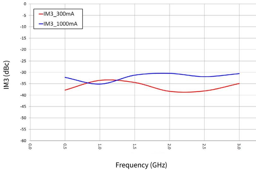
Figure 7. IM3 vs Frequency of the CG2H30070F as Measured in the Single-ended Demonstration Amplifier CG2H30070F-AMP
