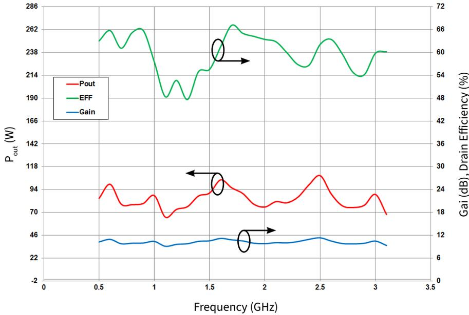
Figure 2. Output Power and Efficiency of the CG2H30070F vs Frequency as Measured in the Single-ended Demonstration Amplifier CG2H30070F-AMP
