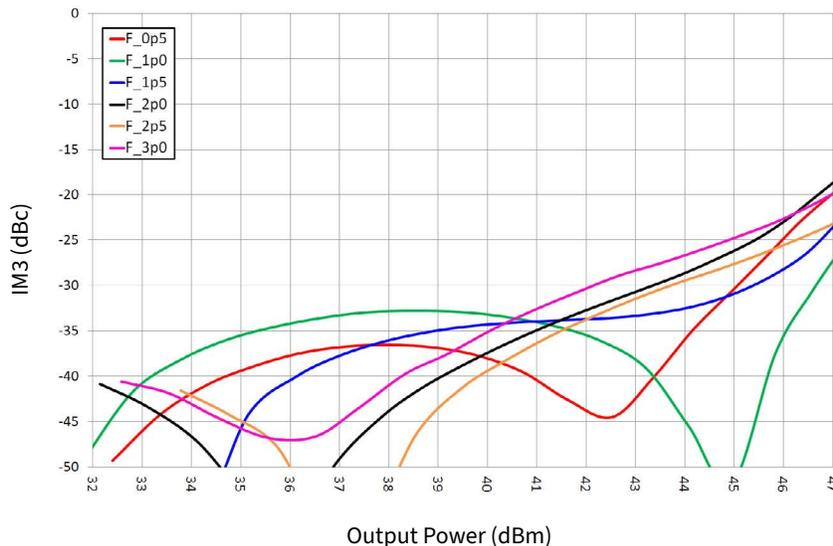
Figure 5. IM3 vs Output Power of the CG2H30070F as Measured in the Single-ended Demonstration Amplifier CG2H30070F-AMP
