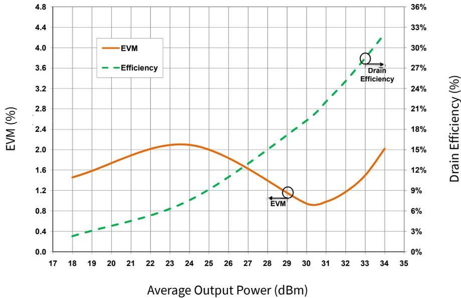
**Figure 3.** Typical EVM and Efficiency of CGH27015 in Broadband Amplifier Circuit at 2.5 GHz
