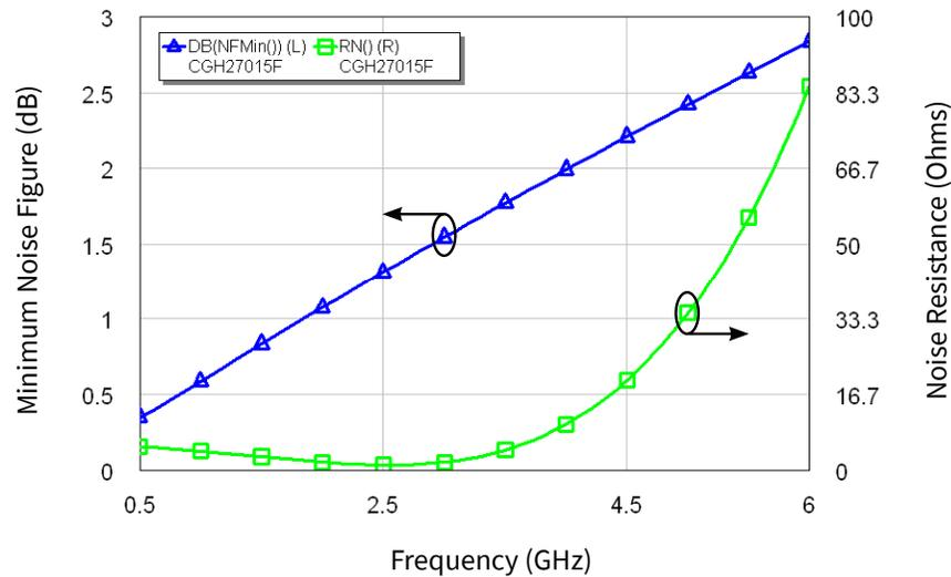
**Figure 5.** Simulated Minimum Noise Figure and Noise Resistance vs Frequency of the CGH27015
