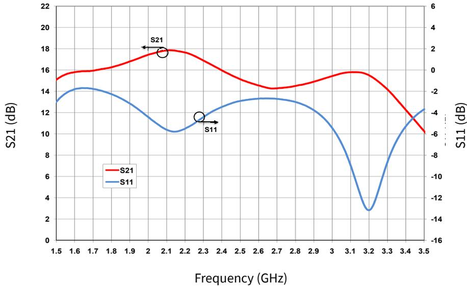
**Figure 1.** Performance of CGH27015 in Broadband Amplifier Circuit
