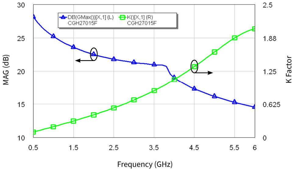
**Figure 4.** Simulated Maximum Available Gain and K Factor of the CGH27015F
