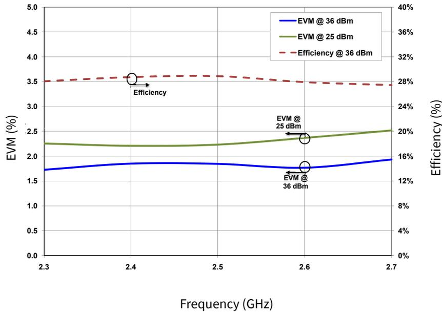
**Figure 2.** Typical EVM and Efficiency versus Frequency measured in CGH27030F-AMP
