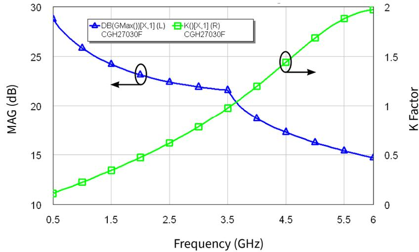
**Figure 5.** Simulated Maximum Available Gain and K Factor of the CGH27030F
