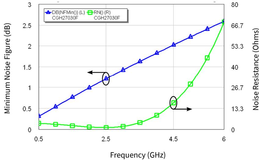
**Figure 6.** Simulated Minimum Noise Figure and Noise Resistance vs Frequency of the CGH27030
