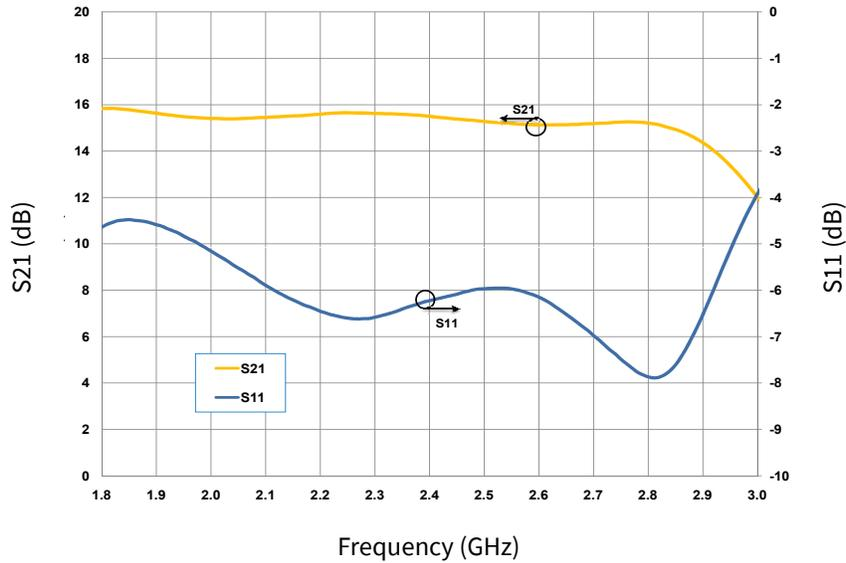
**Figure 1.** Small Signal S-Parameters vs Frequency measured in CGH27030F-AMP
