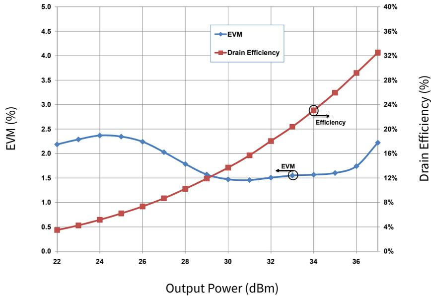
**Figure 3.** Drain Efficiency and EVM vs Output Power measured in CGH27030F-AMP
