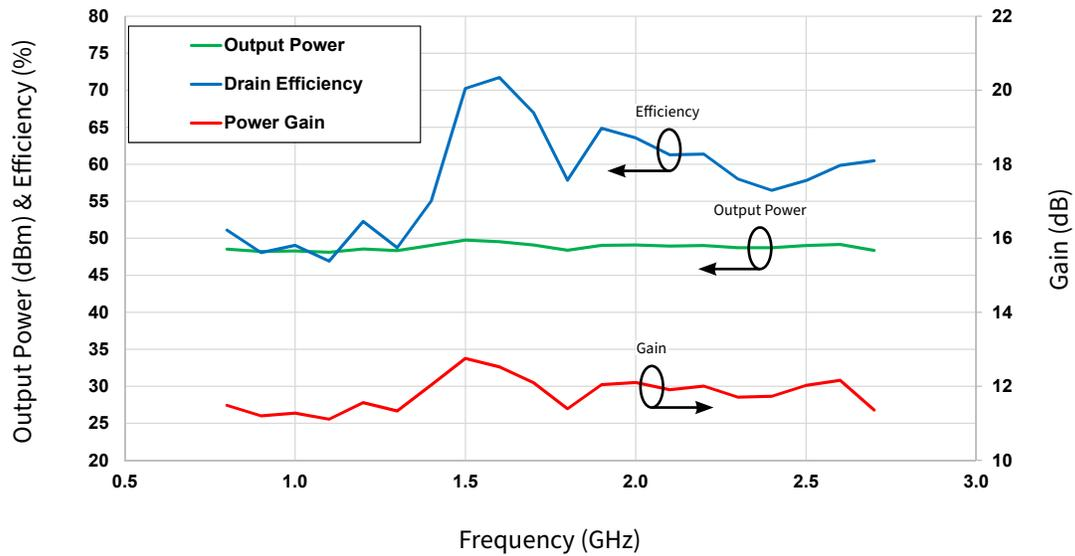
**Figure 4.** Power, Drain Efficiency and Gain vs Frequency of CGHV27060MP-AMP3
