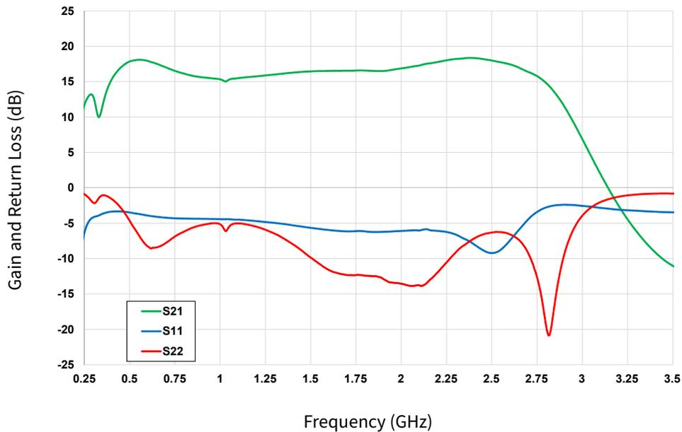
**Figure 3.** Small Signal Gain and Return Losses Measured of the CGHV27060MP Measured in Demonstration Amplifier Circuit CGHV27060MP-AMP3
