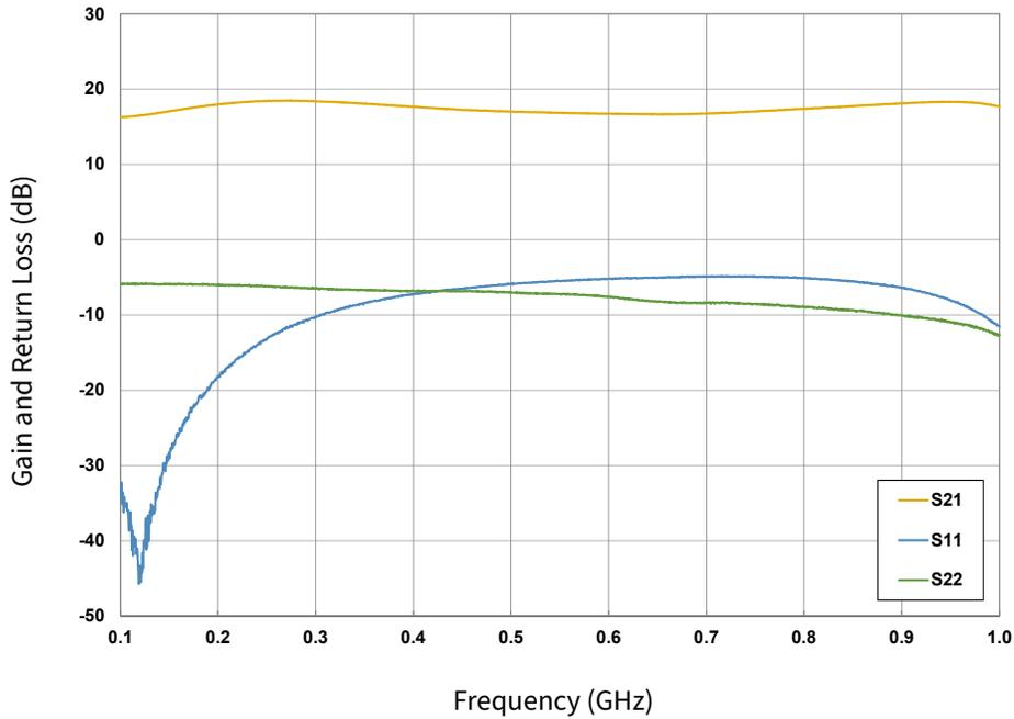
**Figure 5.** Small Signal Gain and Return Losses of the CGHV27060MP Measured in Demonstration Amplifier Circuit CGHV27060MP-AMP4
