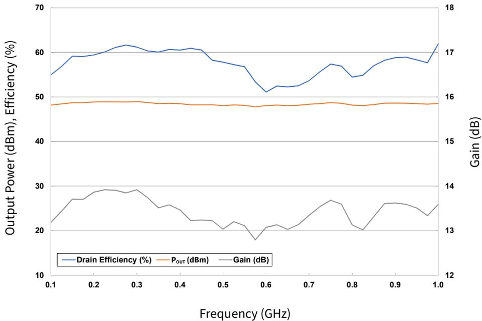
**Figure 6.** Power, Drain Efficiency, and Gain vs Frequency for the CGHV27060MP Measured in Demonstration Amplifier Circuit CGHV27060MP-AMP4
