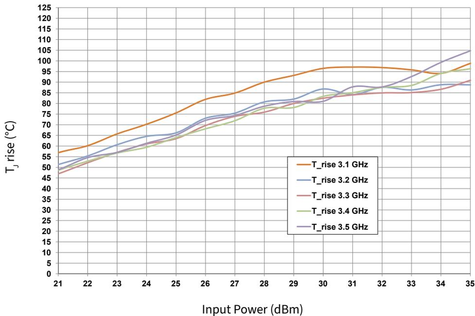
**Figure 5.** CGHV35060MP-AMP1 T<sub>j</sub> rise vs. Input Power
