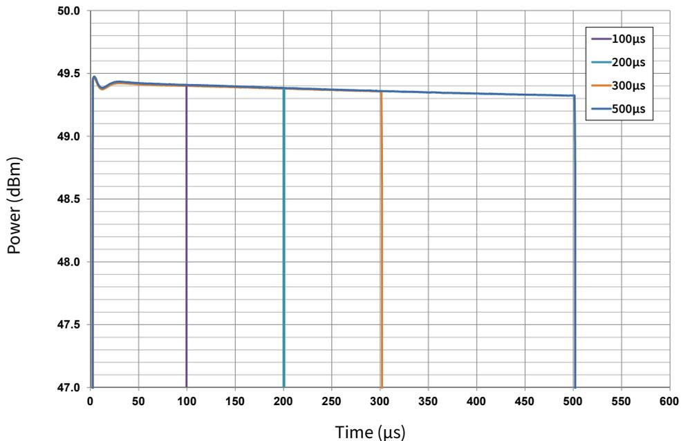
**Figure 6.** CGHV35060MP-AMP1 Output Power vs. Time, Varying Pulse Lengths
