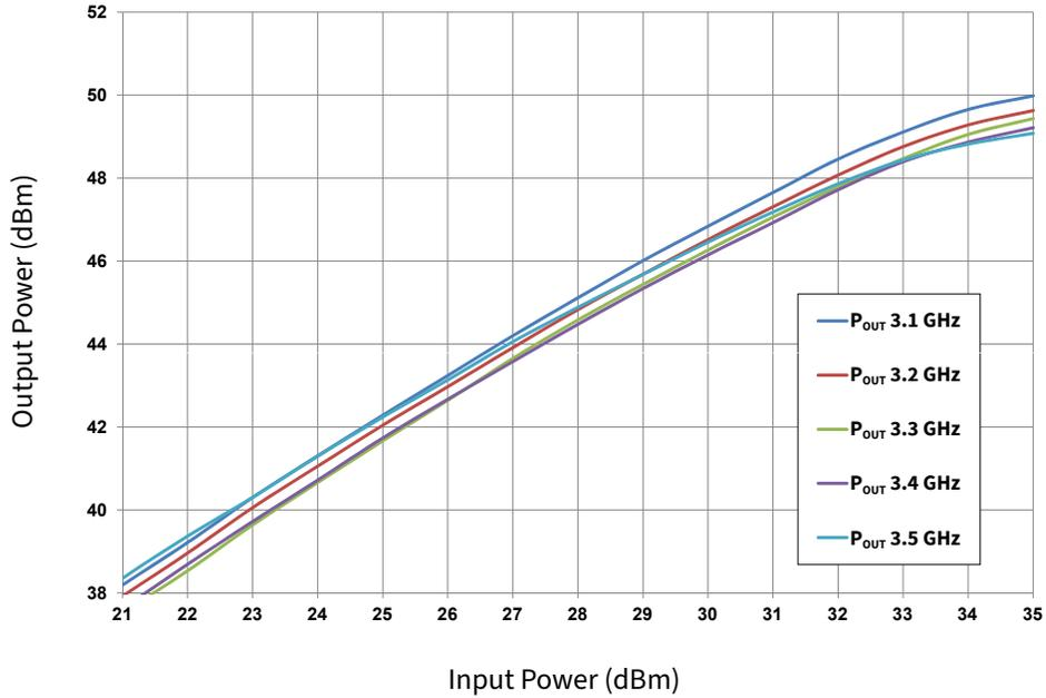
**Figure 3.** CGHV35060MP-AMP1 Output Power vs. Input Power
