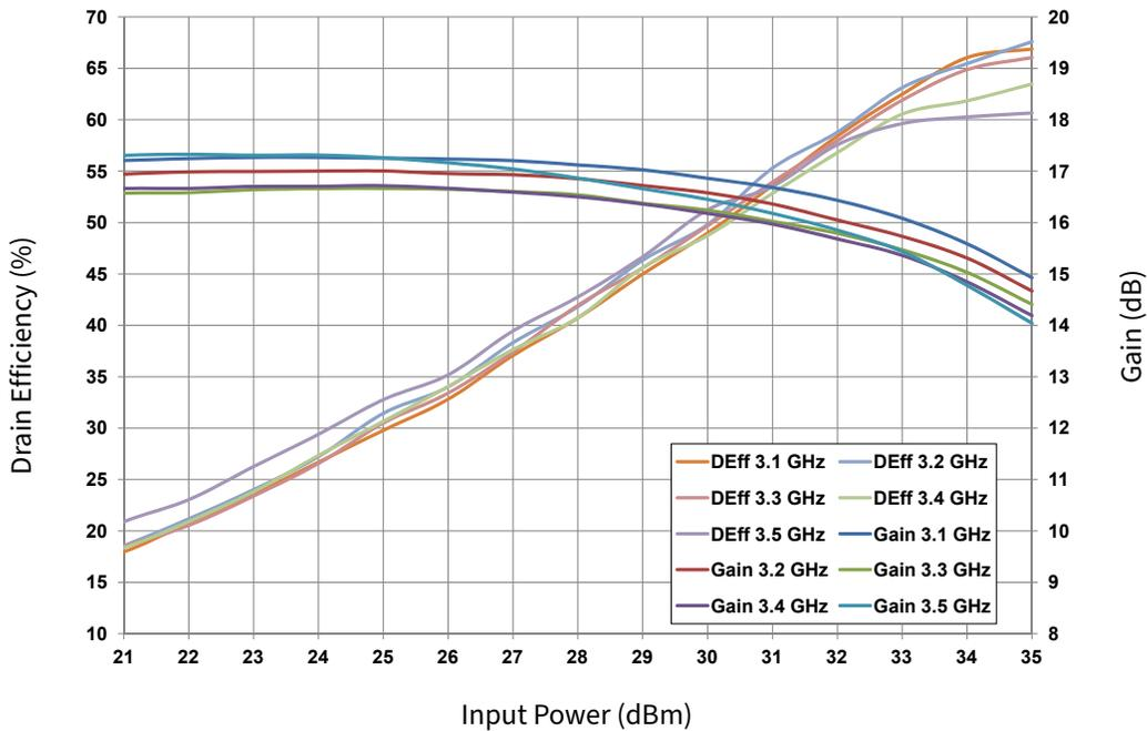
**Figure 4.** CGHV35060MP-AMP1 Gain & Efficiency vs Input Power
