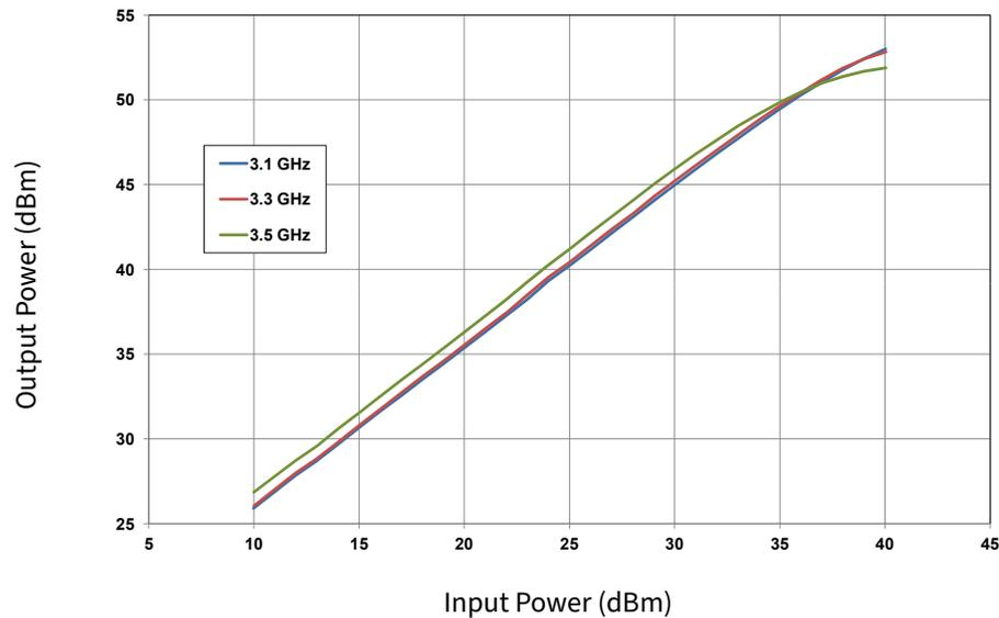
**Figure 3.** CGHV35150 Output Power vs Input Power
