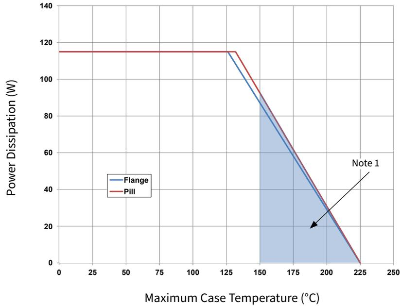
**Figure 5.** CGHV35150 Transient Power Dissipation De-Rating Curve
