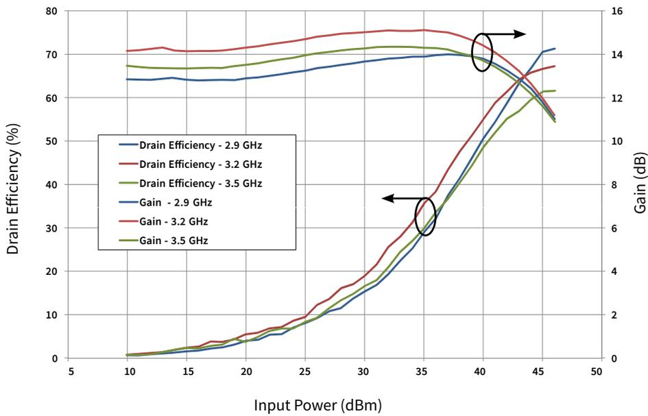
Figure 4. CGHV35400F Drain Efficiency & Gain vs Input Power
