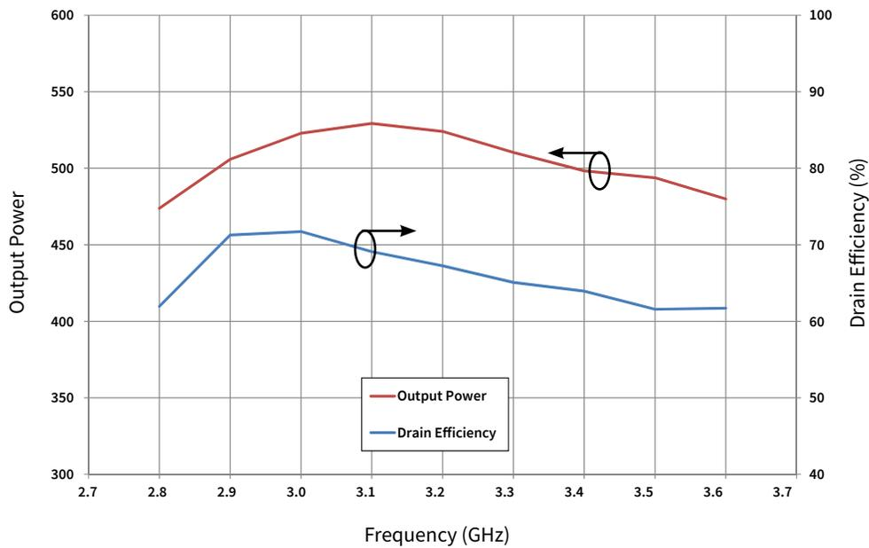
Figure 2. CGHV35400F  $P_{OUT}$  and Drain Efficiency vs Frequency at  $T_{case} = 25\text{ }^\circ\text{C}$
