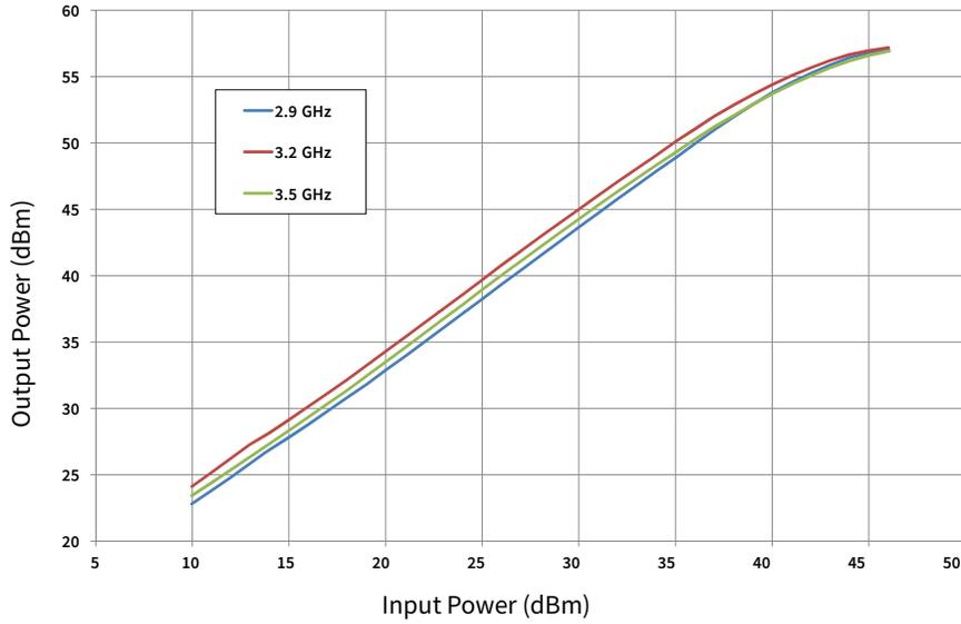
Figure 3. CGHV35400F Output Power vs Input Power
