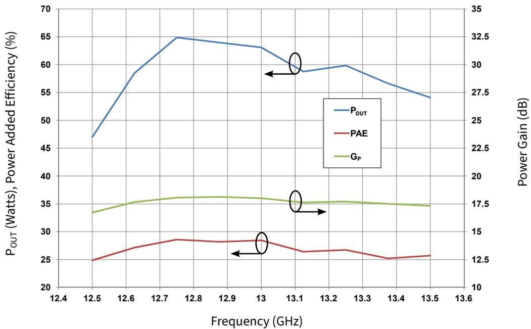
**Figure 2.** Output Power & PAE vs Frequency
