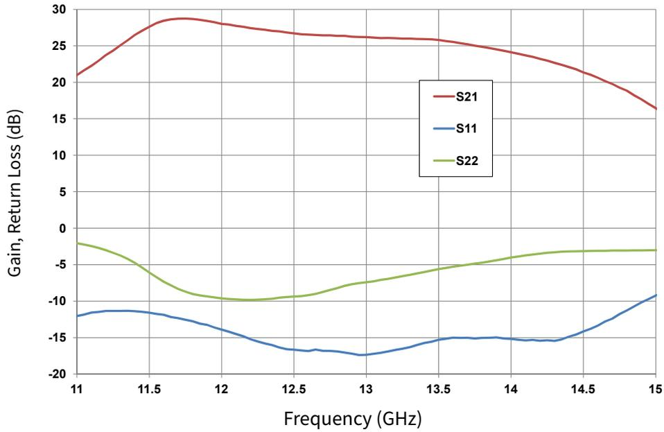
**Figure 1.** Small Signal Gain vs Frequency
