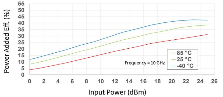
Figure 19. Power Added Eff. vs Input Power as a Function of Temperature
