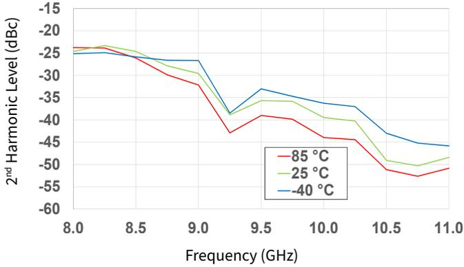
Figure 28. 2<sup>nd</sup> Harmonic vs Frequency as a Function of Temperature
