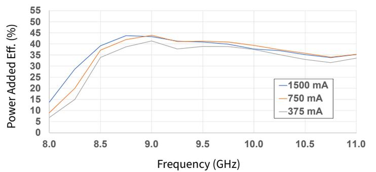
Figure 10. Power Added Eff. vs Frequency as a Function of  $I_{DQ}$
