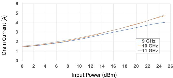
Figure 16. Drain Current vs Input Power as a Function of Frequency
