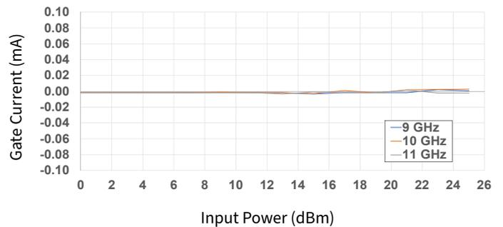
Figure 17. Gate Current vs Input Power as a Function of Frequency
