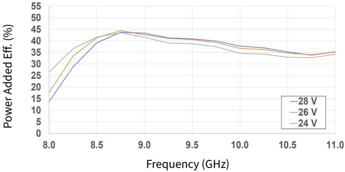
Figure 9. Power Added Eff. vs Frequency as a Function of  $V_D$
