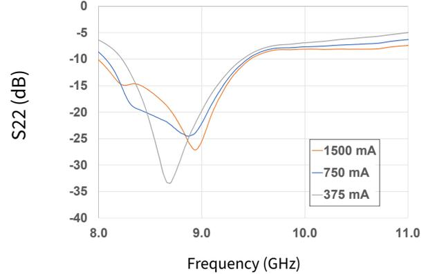
Figure 42. Output RL vs Frequency as a Function of  $I_{DQ}$
