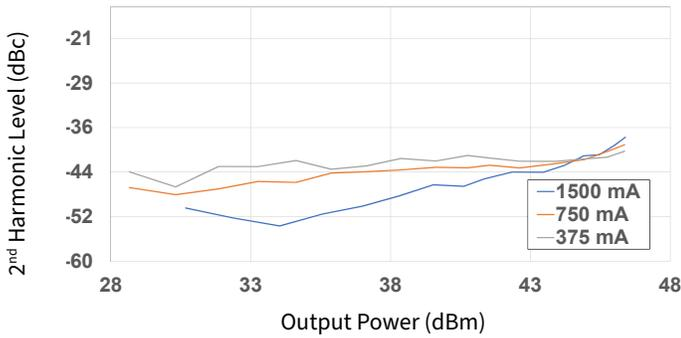
Figure 30. 2<sup>nd</sup> Harmonic vs Output Power as a Function of  $I_{DQ}$
