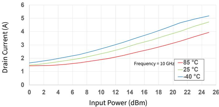
Figure 21. Drain Current vs Input Power as a Function of Temperature
