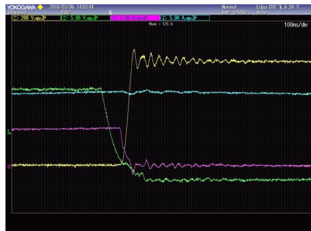
Figure 18. b: MOSFET turn-off waveforms (drain to source voltage ( V_{DS} ) (yellow), gate to source voltage ( V_{GS} ) (green), drain current ( I_D ) (purple) and inductor current ( I_{INDUCTOR} ) (cyan))
