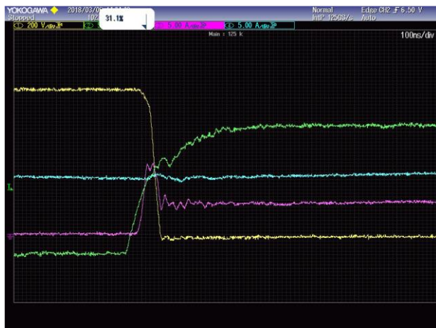
Figure 18. a: MOSFET turn-on waveforms (drain to source voltage ( V_{DS} ) (yellow), gate to source voltage ( V_{GS} ) (green), drain current ( I_D ) (purple) and inductor current ( I_{INDUCTOR} ) (cyan))
