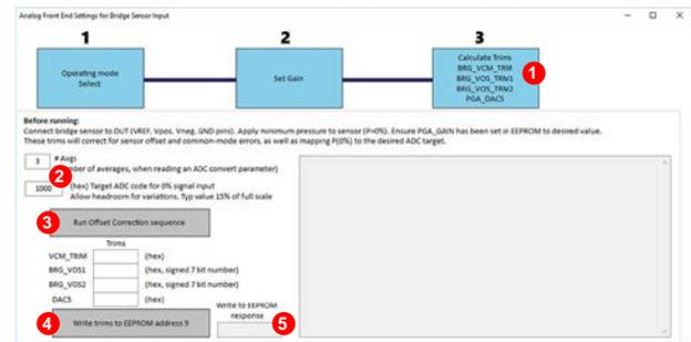
Figure 19. How to Set AFE Trims in the EVAL-ADA4558EBZ Software
