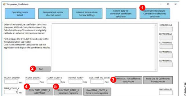
Figure 26. Calibration Window for External Temperature
