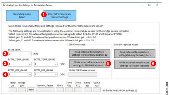
Figure 20. How to Set RTD Gain and Current in the ADA4558EBZ Evaluation Software
