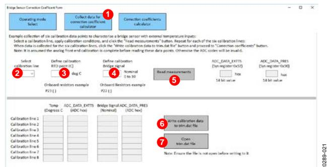
Figure 21. Generate the trim.dat file for the Bridge Sensor Calibration
