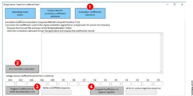
Figure 22. Generate the Bridge Sensor Linearization Coefficients
