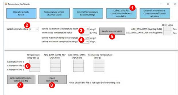
Figure 25. Collect Data for External Temperature Correction Coefficient Calculator
