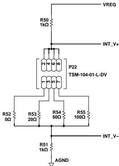
Figure 11. On-Board Test Resistors for the Bridge Sensor Input
