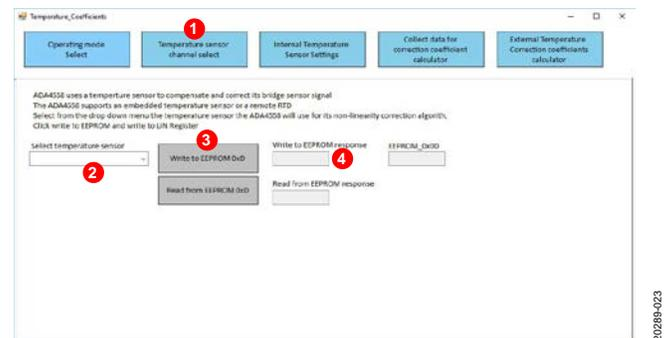
Figure 23. Selecting the Temperature Sensor Channel
