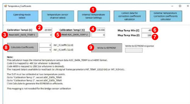
Figure 24. Calibration Window for Internal Temperature
