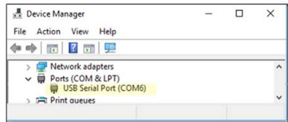
Figure 6. **Device Manager**: Verifying EVAL-ADA4558EBZ Connection to PC
