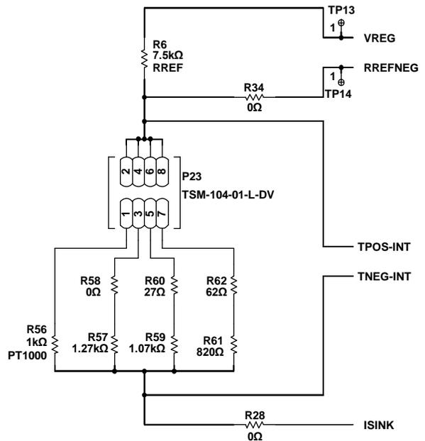
Figure 13. On-Board Test Resistors for the External Temperature Sensor Input
