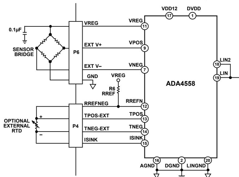
Figure 9. Input Signal Connection Diagram
