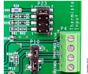
Figure 12. Remote Temperature Sensor Input
