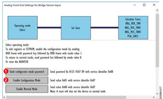
Figure 17. How to Set Configuration Mode in the ADA4558EBZ Evaluation Software
