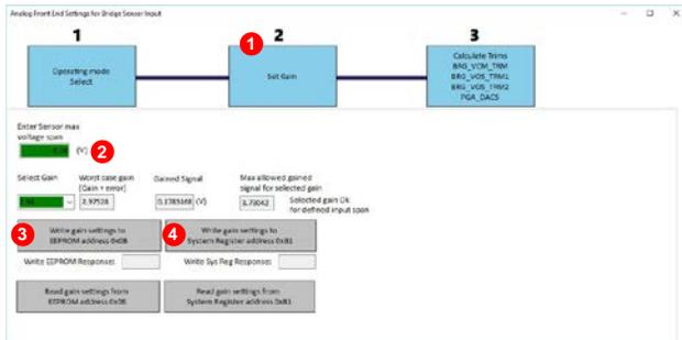
Figure 18. How to Set Gain in the EVAL-ADA4558EBZ Software
