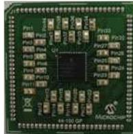
This plug-in module comes with a 44-pin QFN dsPIC33FJ128GP804 device. Plug it into the Explorer 16 board (DM240001).
