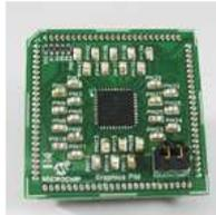
This 100-pin Plug-in Module comes with a dsPIC33FJ128GP804 device in a 44-pin QFN package. Use it as a plug-in module with the Explorer 16 board (DM240001) for development of general purpose DSC control applications.
