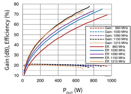
Figure 1. Power Sweep, Pulsed CW
