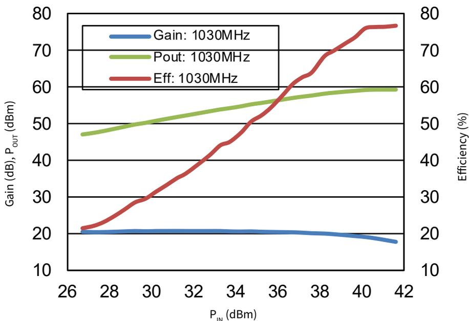
Figure 5. MODE-S: (32  $\mu\text{s}$ -ON/18  $\mu\text{s}$ -OFF) x 48, LTDF-6.4%
