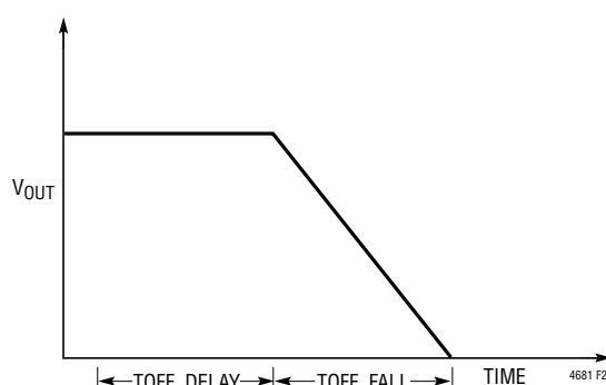
Figure 26. TOFF_DELAY and TOFF_FALL
